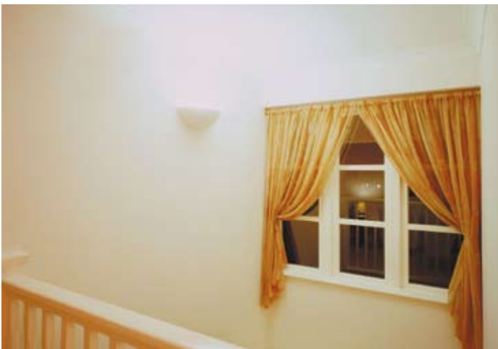
Figure 9 Use of a CFL in a double height space to reduce risk of falls
